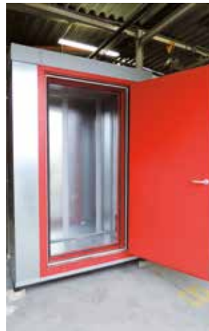
Test specimen in front of the smoke protection chamber
