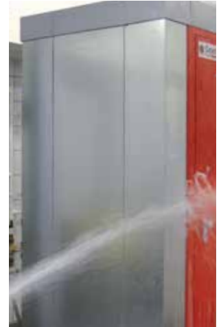
Test against high-pressure water jets
