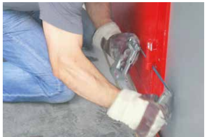
Break-in test: Attack on the hinges
